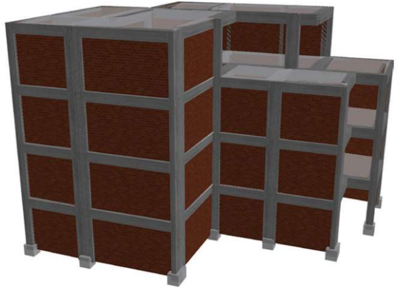
Figure 4.98 Bare and fully infilled building. Source: Stelios Antoniou.
